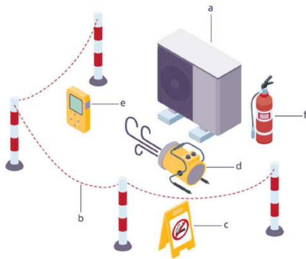
a. Heat Pump b. Bollards c. Safety sign d. ATEX approved fan e. Gas detector f. Fire Extinguisher
